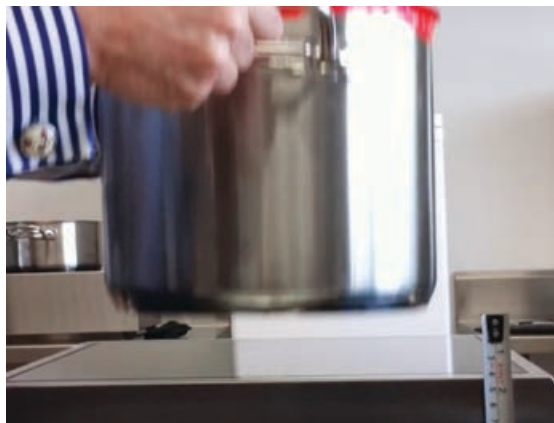
Heavy drop test on tough NEG glass*
